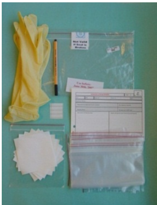
FIG. 10. Environmental swipe sample collection kit.
